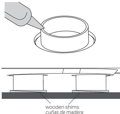
2b. If using mortar, press the shower tray into place while the mortar is still wet. Be sure to apply weight (full water buckets work well) to the tray to ensure proper adhesion. Allow mortar to fully cure before proceeding further.
